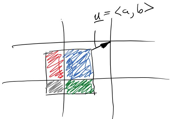
$$\begin{aligned} \underline{u} &= \langle a, b \rangle \\ p_{j,l}^{n+1} &= (1-c_a)(1-c_b) p_{j,l}^n \\ &+ c_a (1-c_b) \boxed{p_{j-1,l}^n} \\ &+ c_b (1-c_a) \boxed{p_{j,l-1}^n} \\ &+ c_a c_b \boxed{p_{j-1,l-1}^n} \end{aligned}$$
