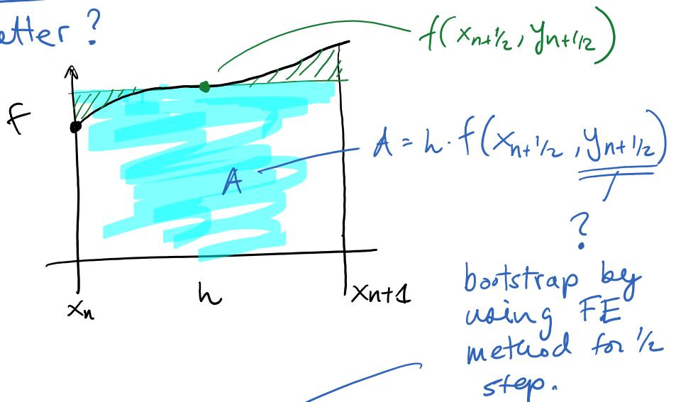
$$y_{n+1/2} = y_n + \frac{h}{2} f(x_n, y_n) \quad \begin{matrix} \text{use this} \\ \text{in the} \\ \text{integral} \end{matrix}$$
